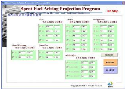
Figure 3. The third step window for input of the cycle length and the batch size of NPPs
