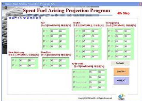
Figure 4. The fourth step window for input of the discharge burn-up and the capacity factor of NPPs
