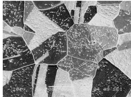
Fig. 1. The microstructure of the alloy 600 etched in a Bromine Methanol solution. Magnification: x500.
