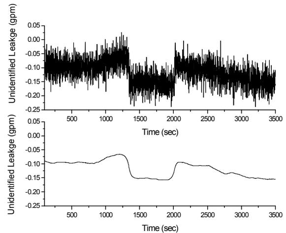
Figure 2. Unidentified leak rate using a conventional technique (upper) and a Kalman smoother (lower)
