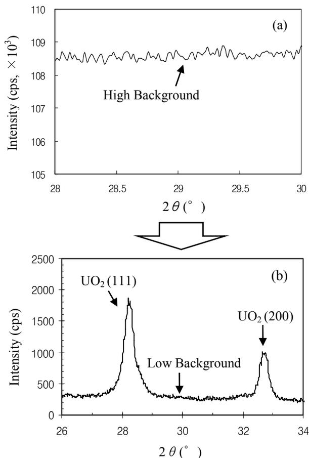
Figure 2. Comparison of background intensity for a spent fuel before (a) and after (b) detector shielding.
