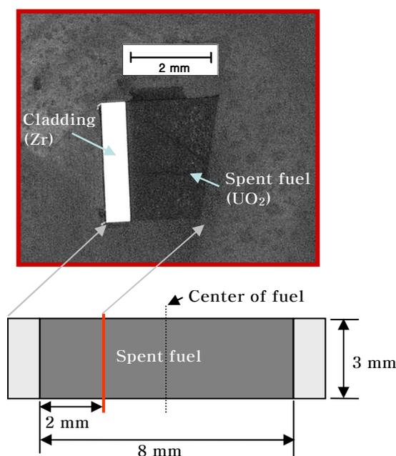
Figure 1. Spent fuel discharged from Yeonggwang-2 PWR reactor. (Burn up 55000 MWd/MtU)
