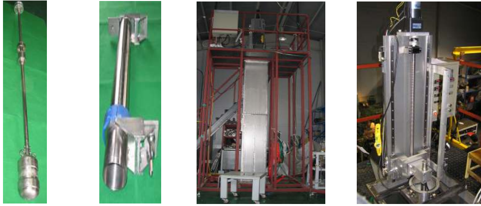
a. Dummy weight b. Damping Mechanism c. Test pool d. Drive mechanism
