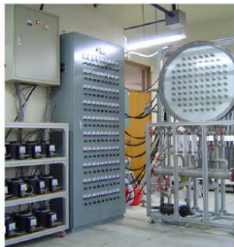
Fig.1 HUKINS-1/8 scale Moderator cooling system [1]
