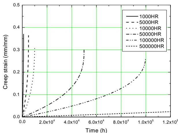
Fig. 5. The long-term creep curves predicted for alloy 617 at 950°C.
