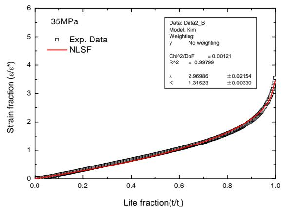
Fig. 2. Strain fraction vs. life fraction curve obtained by NLSF of the modified K-R equation at 35MPa.
