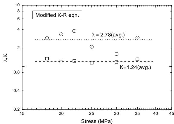
Fig. 4. A stress dependency of the  $K$  and  $\lambda$  in the modified K-R model.
