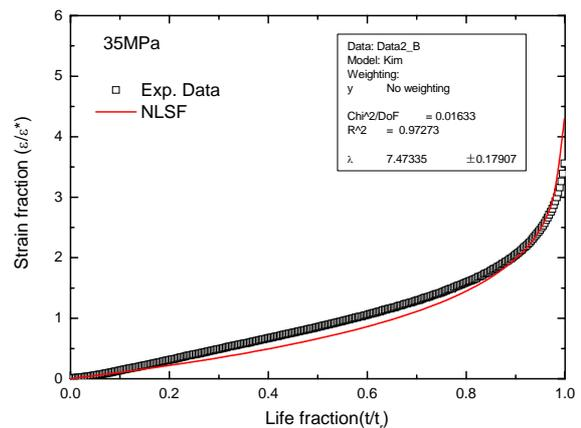
Fig. 1. Strain fraction vs. life fraction curve obtained by NLSF of the K-R equation at 35MPa.
