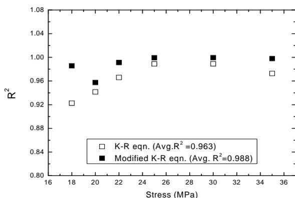
Fig. 3. Comparison of the  $R^2$  values between the K-R and modified K-R models.
