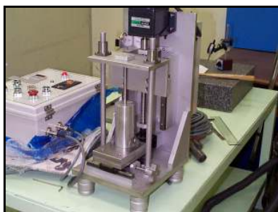
Figure 2. Specimen disassembling from specimen holder by specimen press machine installed in M5a hot cell.
