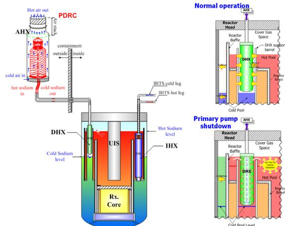
Figure 1. Overview of the PDRC System
