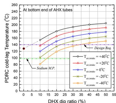
Figure 2. PDRC cold-leg temperature variations
