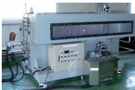
Fig. 1. A Mock-up for Testing Ultrasonic Cleaning of a Nuclear Steam Generator
