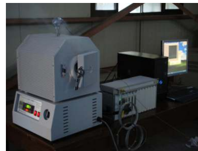
Figure 2. Thermal characterization test equipment.
