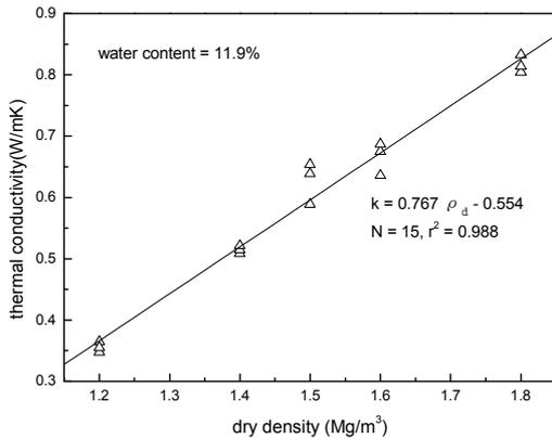
Fig. 1. Thermal Conductivity versus Dry Density of Bentonite (water content = 11.9%)
