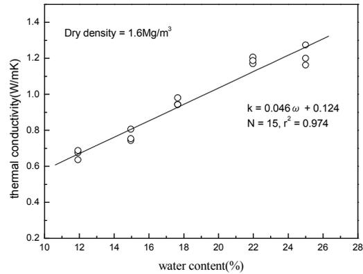
Fig. 2. Thermal Conductivity versus Water Content of Bentonite (dry density= 1.6  $Mg/m^3$ )
