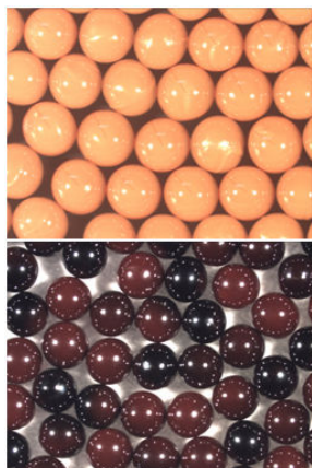
Fig.3. ADU gel and UO_3 particles obtained in our experiment.
