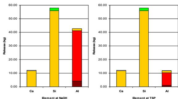
Figure 1. Release from sump using containment spray additive as NaOH(left) and TSP(right) for 24 hours.
