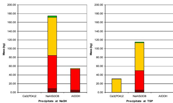
Figure 2. The amount of precipitation using containment spray additive as NaOH(left) and TSP(right) for 24 hours.
