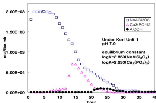
Figure 3. The trend of settling rate under TSP(without Cal-Sil) based on Kori Unit 1.
