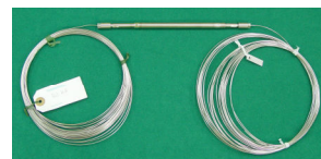
(b) The dual instrumented fuel rod to measure the center and surface temperature of nuclear fuel
