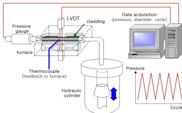
Fig. 1 The cyclic pressurization device designed for the fuel cladding
