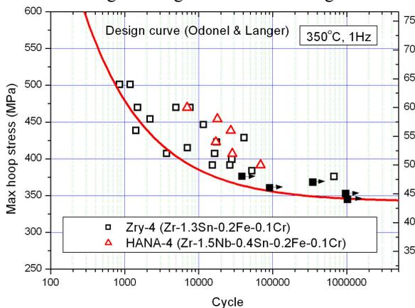
Fig. 2 Stress-life diagram of zirconium cladding with the loading frequency. (Closed symbol with an arrow mark indicates that specimen did not rupture after a given cycle.)
