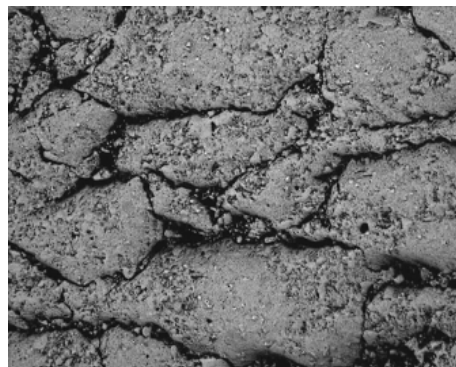
Fig. 2 Microstructures of Dy_xZr_yO_z pellet sintered by using previous process.
