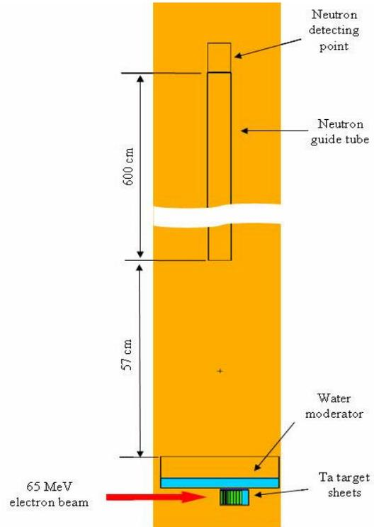
Figure 2. Geometrical model for the target system and neutron guide tube used in the MCNPX simulation
