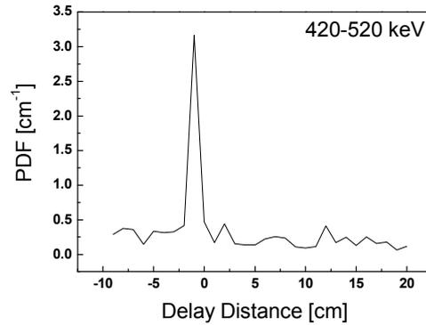
Figure 5. The resolution function for the energy range from 420 to 520 keV
