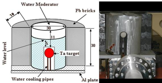
Figure 1. Ta-target system
