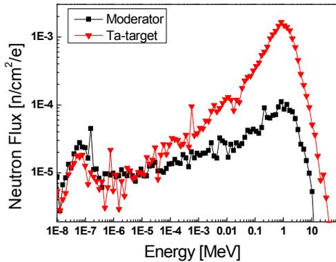
Figure 3. The neutron spectra at surfaces of the Ta-target and the water moderator
