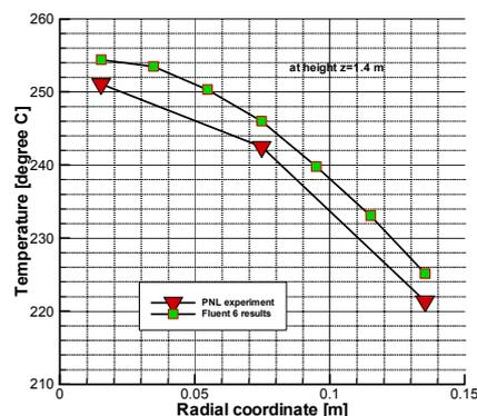
Figure 3. Radial temperature distribution
