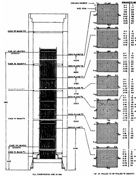
Figure 1. Schematic of the test section
