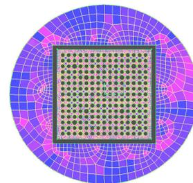
Figure 2. Mesh formation of 15x15 fuel assembly
