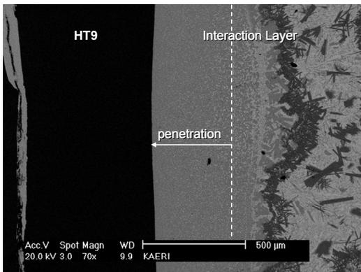
Figure 2. A scanning electron micrograph of a U-10Zr vs. HT9 diffusion couple annealed at 800°C for 7 hours.
