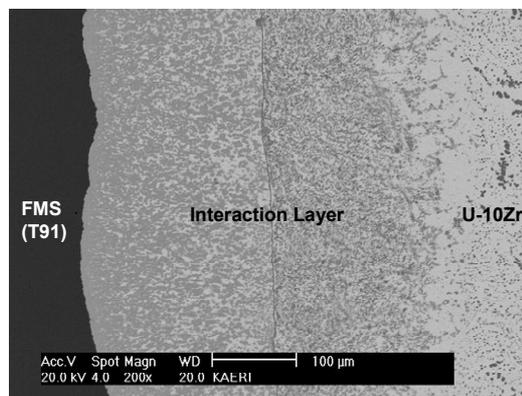
Figure 1. A scanning electron micrograph of a U-10Zr vs. T91 diffusion couple annealed at 740°C for 25 hours.
