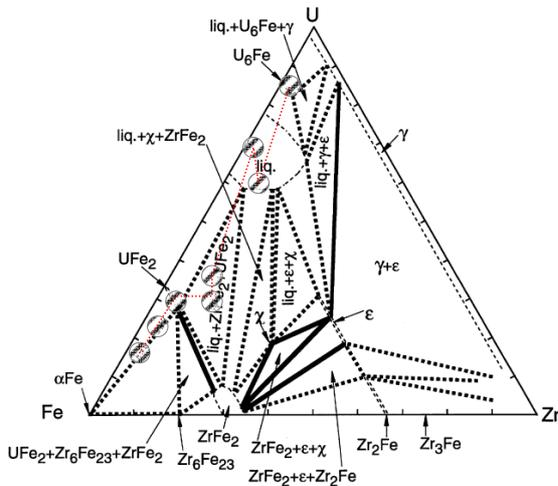
Figure 3. Ternary phase diagram of U-Zr-Fe at 800°C proposed by Nakamura et al.[5]. A diffusion path obtained in this study was superposed.
