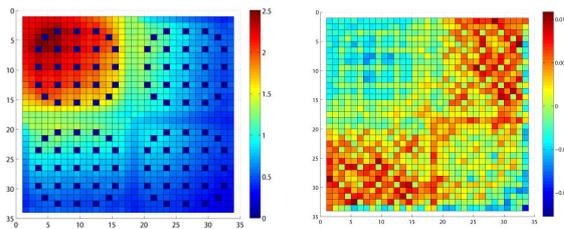
(a) Pin power distribution (b) Pin power error distribution
