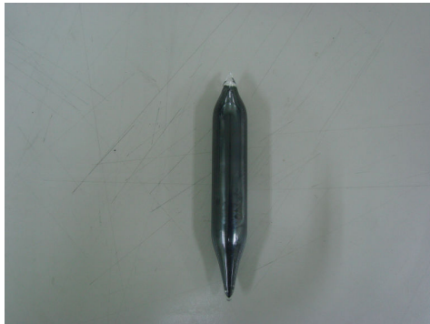
Fig. 3 Vacuum sealed ampule for the crystal growing
