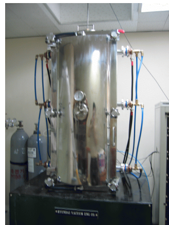
Fig. 1 3-Zone Bridgman Furnace for crystal growing
