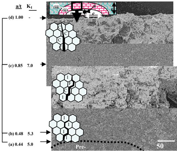
Fig. 1. Fractographs and fracture modes of an ISCC crack for the re-crystallized Zircalloy-4 cladding pressurized in an iodine environment at 350°C; (i) Fatigued pre-crack, (ii) ISCC (iii) ductile fracture after test; I=IG, C= TG by cleavage, F=TG by fluting .
