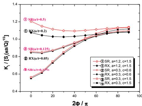
Fig. 2. Typical results of the stress intensity factors for the surface crack formed by the GBPC mechanism on the SR and RX grain surfaces.
