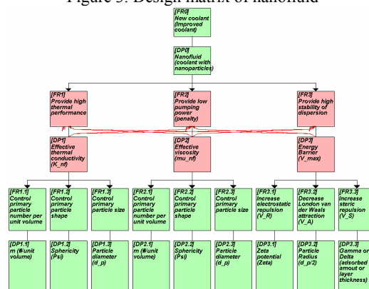
Figure 4. Hierarchical tree of nanofluid design
