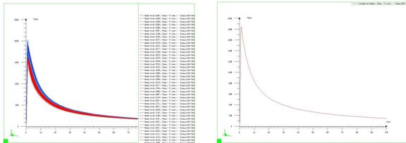
a) Extracted thermal cycle b) Averaged thermal cycle
