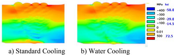
Figure 8. Axial stress results of different cooling rate
