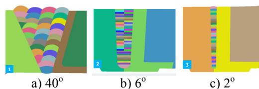
Figure 3. Different Joint Angles and bead shapes for DVI Nozzle
