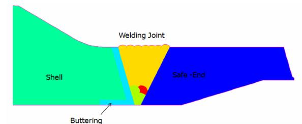
Figure 2. A schematic design of DVI Nozzle welding joint
