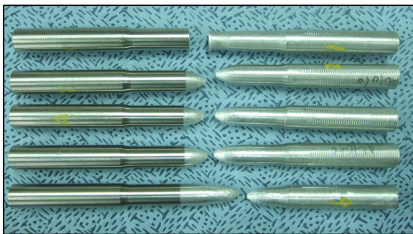
Figure 4. Appearance of the fractured tensile testpieces.
