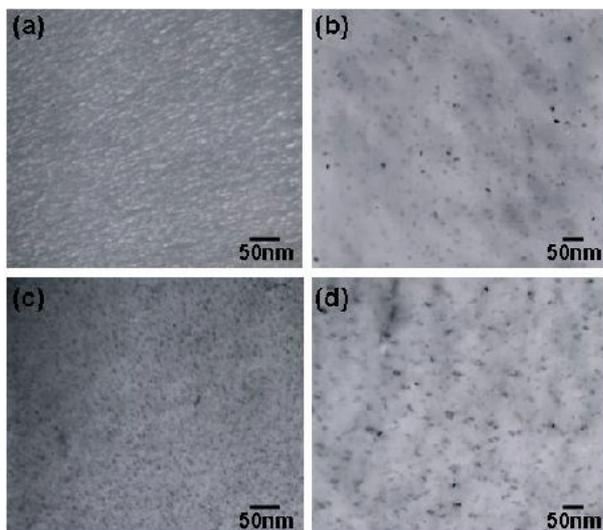
Figure 1. TEM (a) dark and (b, c, d) bright field images of the CuCrZr alloys which were cooled by (a, b) the water quenching and (c, d) the rapid gas cooling after solution annealing at 980°C for 0.5h and then aged at (a, c) 440°C and (b, d) 580°C for 2h.
