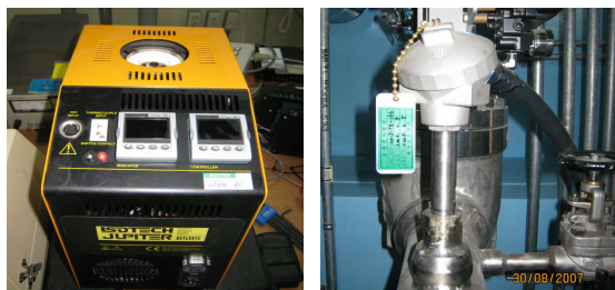
Figure 1. Dry block and Installed RTD
