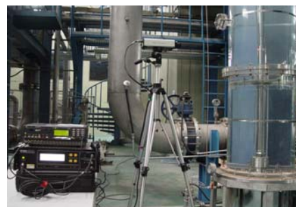
Figure 3. Single channel out-pile test loop and Laser Doppler Vibrometer.
