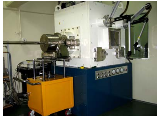
Fig. 1. Radiation shielded glove box and cask adapter for laser ablation system
