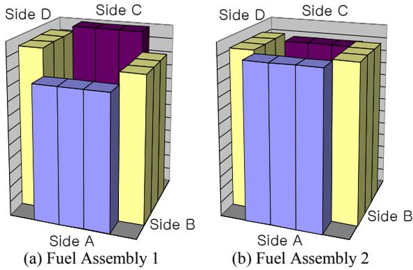
Fig. 1. Fuel assembly growth at each side of the fuel assemblies
