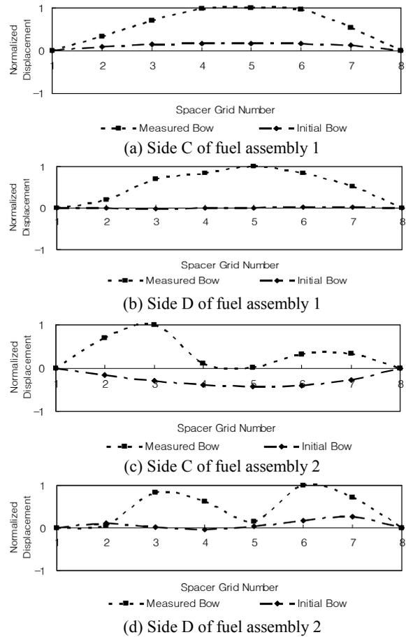
Fig. 3. Fuel assembly bow
