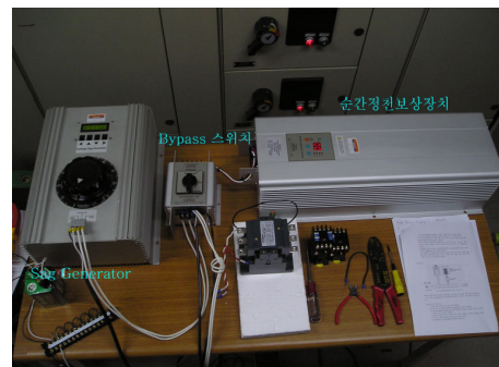
Figure 2. Test setup for impact of momentary interruption on SOR
