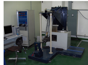
Fig. 1. Layout for Spacer Grid Crush Test Equipment
