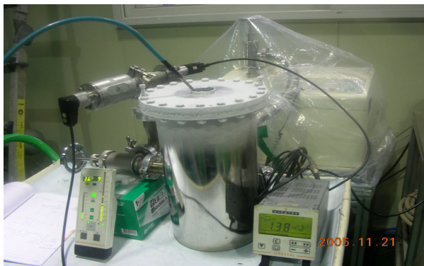
Figure 1. Cryogenic leak test of moderator cell at 77 K
