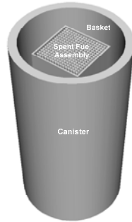
Figure 1. Schematic of the prototype single spent fuel storage unit
