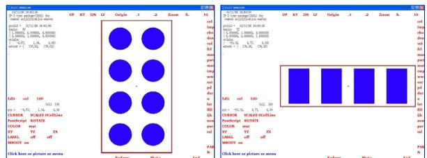
Figure 1. Vertical & horizontal schematics of MCNP analysis
