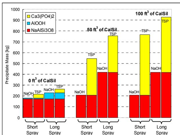
Fig. 2 Comparison of the chemical precipitates with various plant environments.
