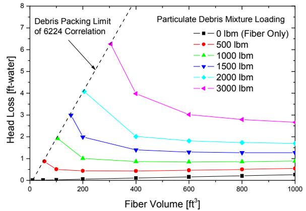
Fig. 1 Head loss with various mixed debris loading on the 1000 ft<sup>2</sup> sump screen (7000 gpm ECCS flow).
