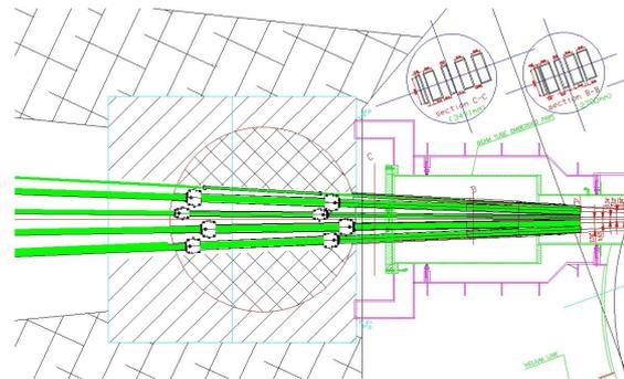
Figure 2 Conceptual layout of main shutter
