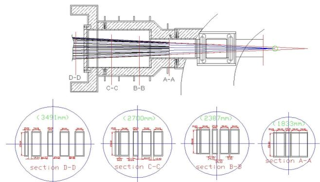
Figure 1 The conceptual layout of in-pile guide channel
