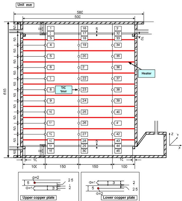
Figure 1. SIGMA RP heater and thermocouple locations.
