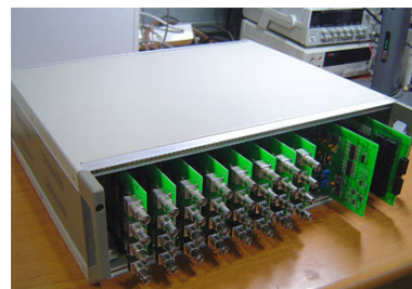
Fig.3 The axial tomography analyzer for data acquisition and electrodes switching.
