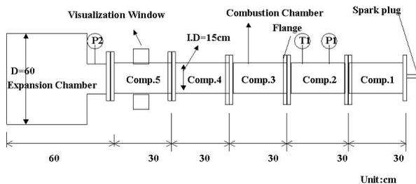
Fig. 1 Combustion chamber
