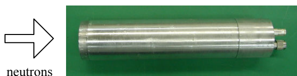
Figure 1. A tube detector with very thin wire hold block for FCD.
