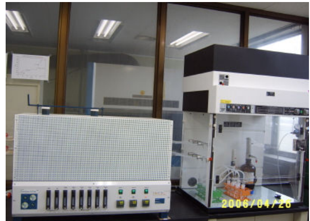
Fig. 2. The combustion furnace with auxiliaries for oxidizing the samples
