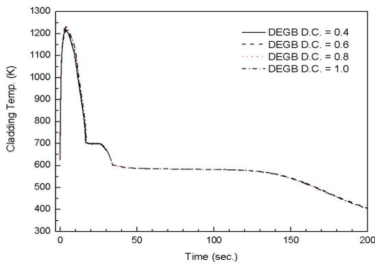
Fig. 1. PCT for the Double-Ended Guillotine Breaks of Pipes
