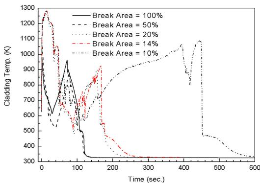
Fig. 2. PCT for the Longitudinal Splits of Pipes
