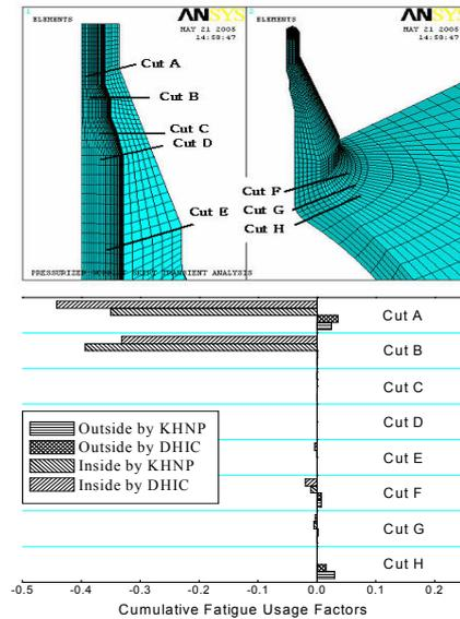
Figure 5. Cumulative fatigue usage factors at cut location of CVCS charging nozzle.
