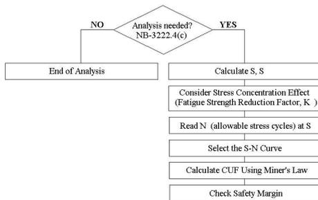
Figure 1. Procedure of ASME fatigue analysis.
