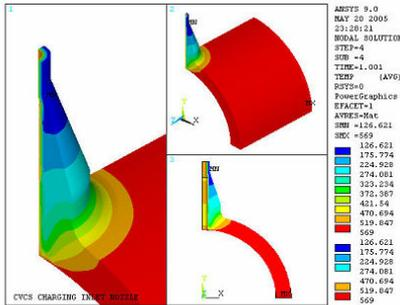
Figure 3. Thermal distribution of CVCS charging nozzle.
