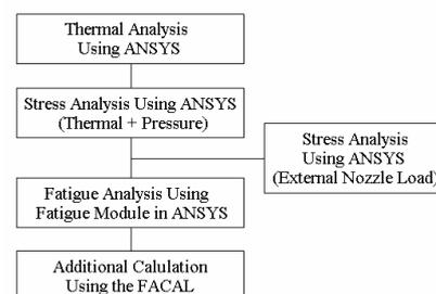
Figure 2. Fatigue analysis using ANSYS and FACAL code.
