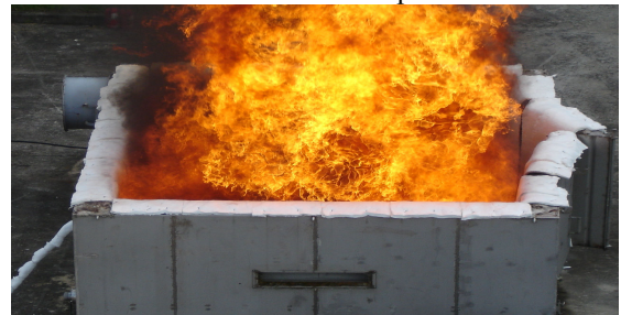
Figure 6. Fire test under 800°C flame temperatures and 30 minutes
