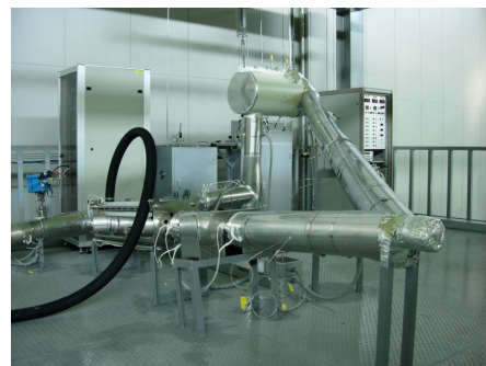
Fig. 2. The photograph of lead corrosion test loop at KAERI (KPAL-II)
