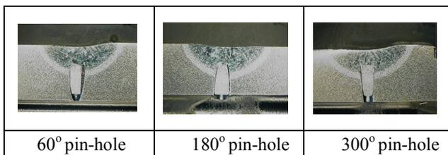
Fig. 4. Macro-sections of the pin-hole welded specimens.
