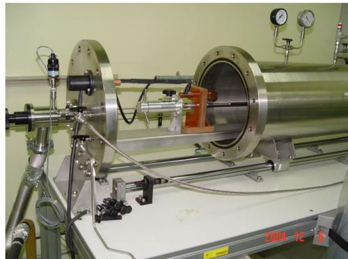
Fig 2. Photography of the GTA welding chamber.
