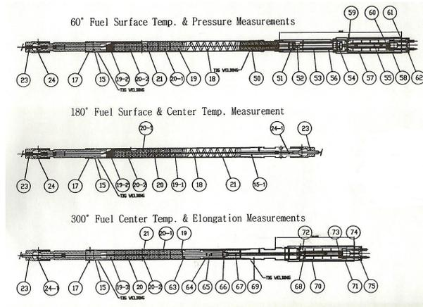
Fig 1. Configuration of the dual rod specimens.
