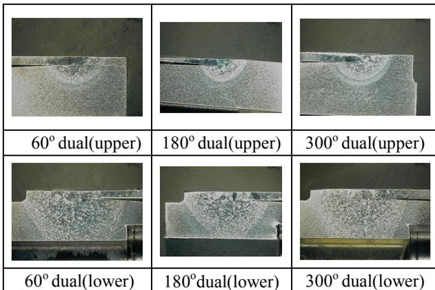
Fig. 3. Macro-sections of the upper and lower sides with dual rod specimens.
