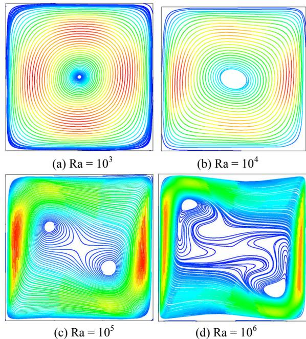
Figure 1. Streamlines predicted by predicted by using CFX-10, with 80X80 meshes
