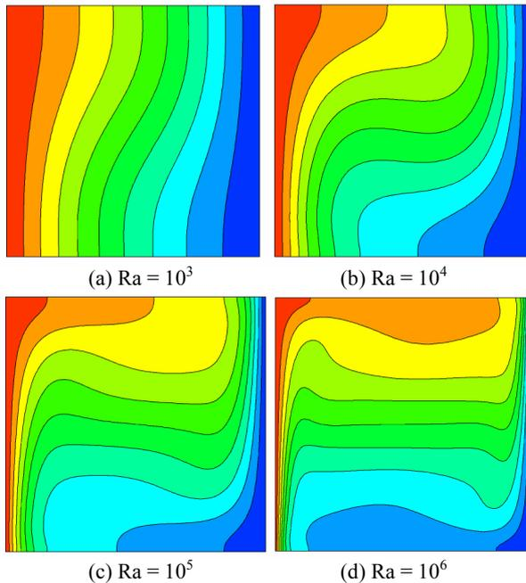
Figure 2. Contour maps of temperature predicted by using CFX-10, with 80X80 meshes
