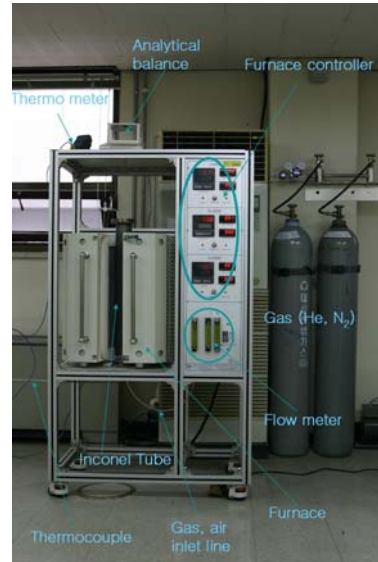
Figure 1. Test System for graphite oxidation
